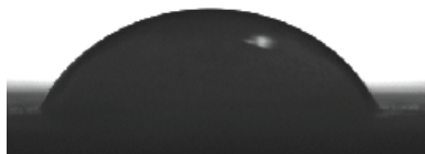
Water droplet on painted surface with conventional paint Contact angle: 60°
